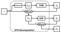
Figure 3.5. Illustration of the Three-Component Image Decomposition Algorithm
