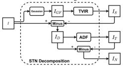
Figure 2.1. Diagram of image decomposition into three components
