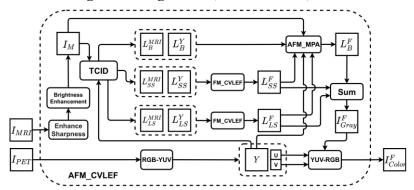
Figure 3.6. Proposed image fusion diagram
